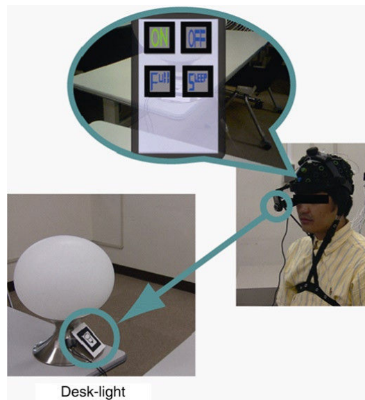
Figure 1.32 – An AR system allowing users to look at various appliances and sending commands to them using a BCI [Kansaku, 2011].
