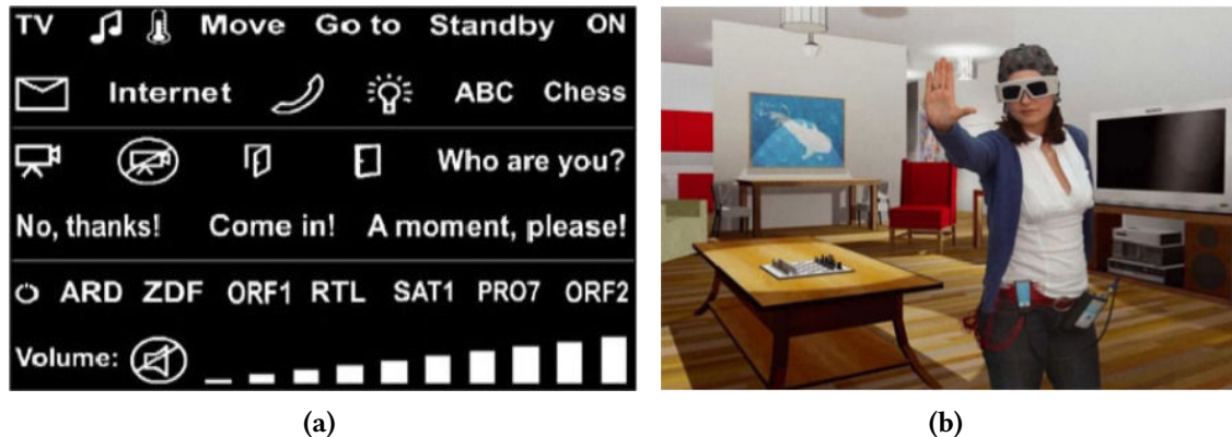
Figure 1.24 – Home automation in VR driven by P300 and SSVEP. (a) A TV control mask, selection was achieved using the P300 paradigm. (b) Person issuing a command in the virtual environment [Edlinger et al., 2011].
