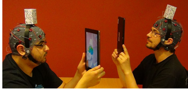
Figure 3.13 – Multi-user visualization of brain activity: two users are visualizing each other's brain activity in real-time using two tablet PCs.
