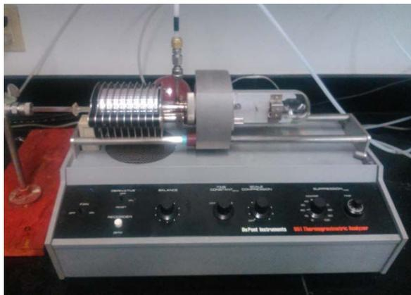
Figure II-13: Dupont Thermogravimetric Analyzer (TGA) used for methane cracking tests over a bed of biochars
