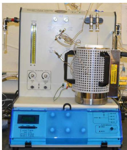
Figure II-8: Chembet Pulsar TPD instrument from Quantachrome company
