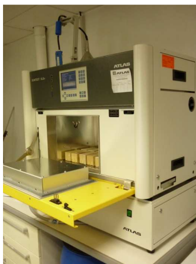
Figure 5.1: Atlas Suntest XLS+ weathering chamber
