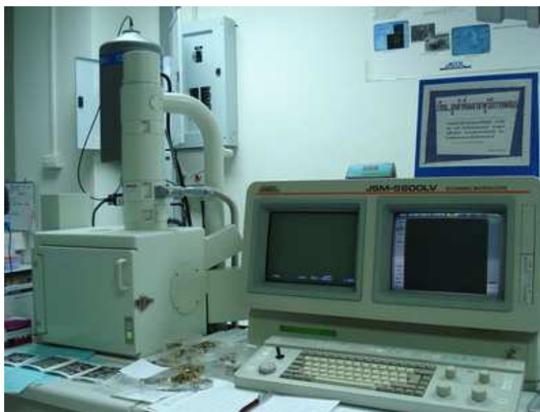
Figure 2-6 Scanning electron microscope scheme (left) and machine (JSM-5800LV) (right)
