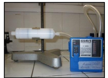
Fig.1: URG personal sampler
