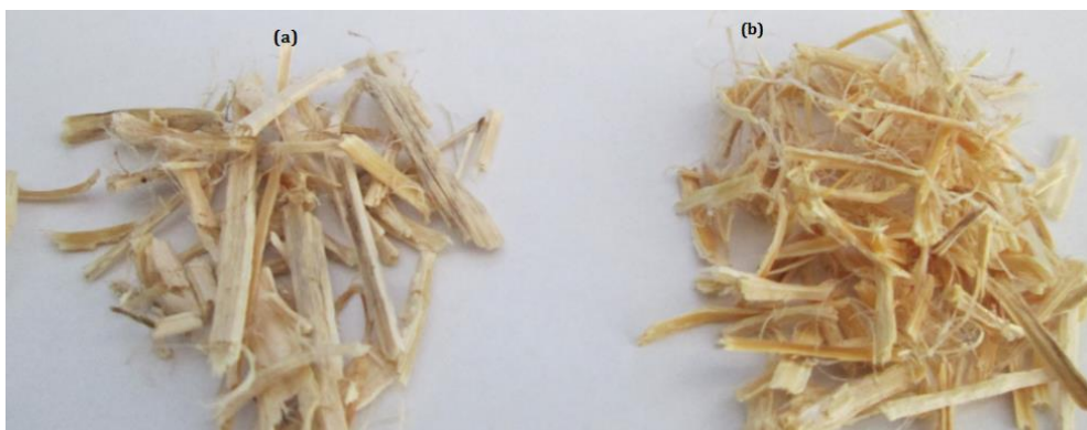
Figure 6: Influence du traitement silane (a) SS1, (b) SS6.
