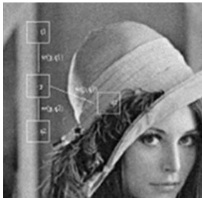
Figure 2.2-5 NL-Means algorithm principle: similar pixels in similar blocks will have a larger weight in the final filtering
