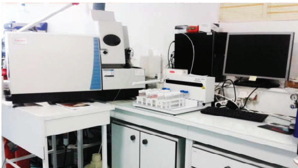
Figure 26 ICP-MS system consisted of an injector, a pump, an inductively coupled plasma mass spectrometer, a collision cell, a detector, and a computer system.
