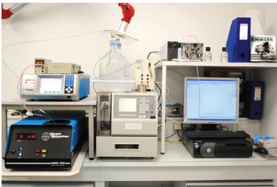
Figure 21 SEC-MALS system; consisted of an online degasser, an injector, a pump, 3 chromatographic columns with a guard column, a refractive index detector, a multi-angle light scattering detector, and a monitor.
