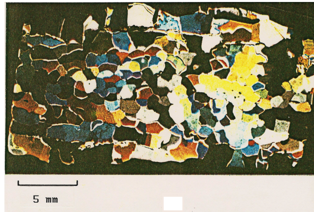
Figure 4.2: Grain boundaries in atmospheric ice accumulated at -4.8^{\circ}\text{C} [100]
