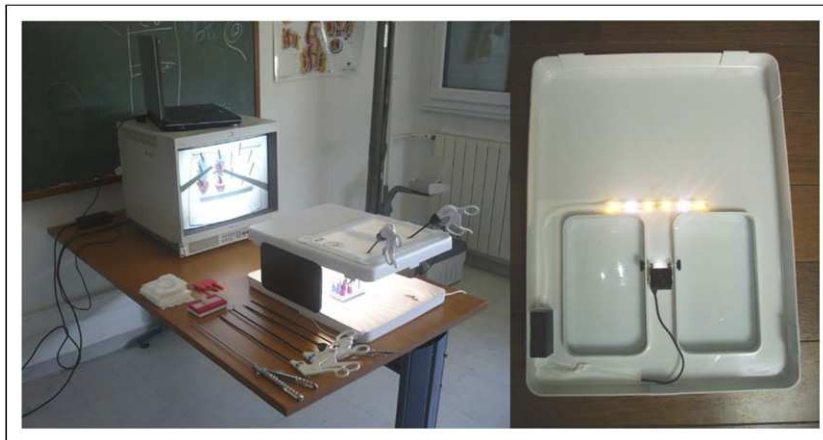
Figure 2 MISTELS Simulator. On the right is the superior part of the box with camera and light-emitting diodes.
