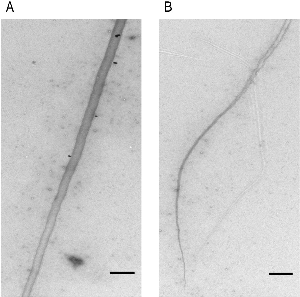
The fiber has cylindrical architectures, with two ends, (A) is the thick end and (B) is thinner; the scale bar is approximated as 200 nm.
