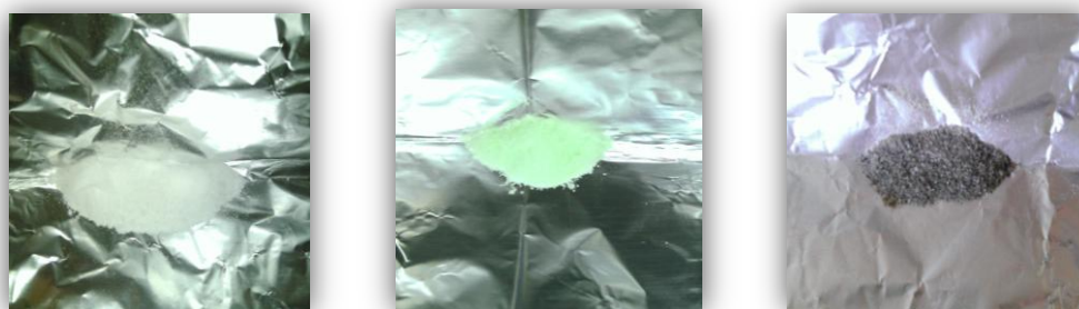
Figure 3.16: Photographic images of the samples SiO 2 (a), Ni salt@SiO 2 (b), Ni(200°C)@SiO 2 and Ni(400°C)@SiO 2 (c).
