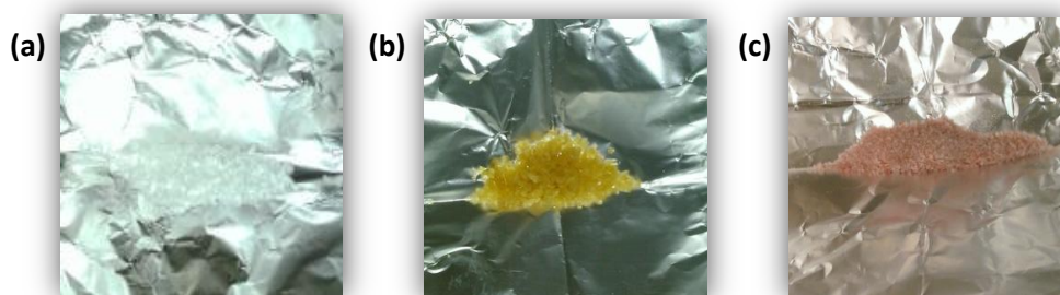
Figure 2.3: Photographic images of the samples Silica (a), Ag@Silica (b) and Au@Silica (c).
