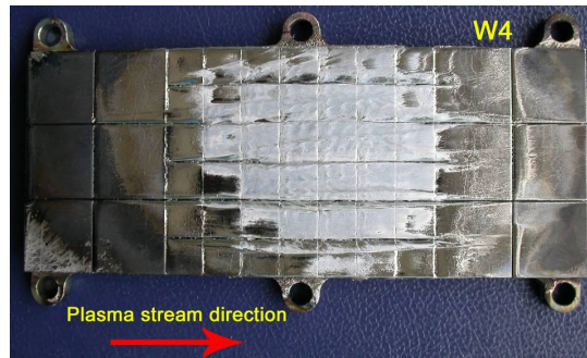
Figure 1.14: Melted Tungsten divertor after an ITER-like ELM. Picture from [Linke 2007].
