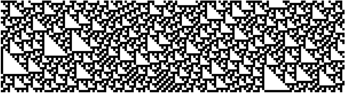
Figure 0.8: The elementary CA F_{102} , starting from an initial configuration drawn randomly according to a Bernoulli measure of parameters (\frac{1}{3}, \frac{2}{3}) .
