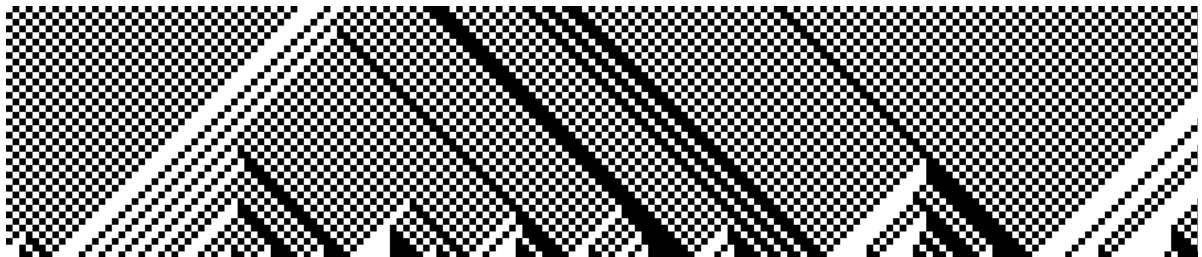
Figure 0.4: Space-time diagram of the traffic automaton from an initial configuration drawn uniformly at random.
