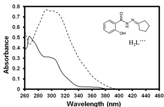
**A5:** Absorbance spectra of H<sub>2</sub>L' (dotted line) and H<sub>2</sub>L''' (thin line), both at 5 · 10<sup>-5</sup> M
