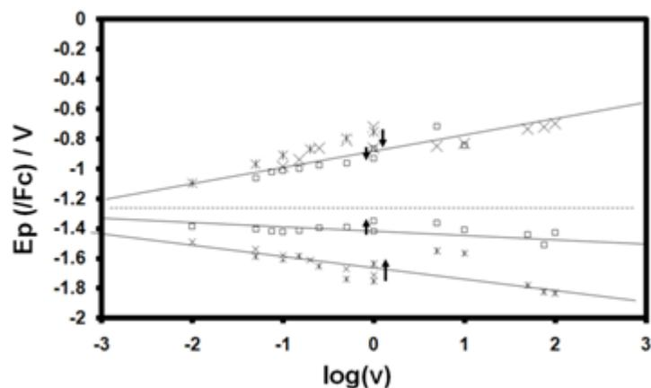
A 12: Plot of  $E_p$  vs.  $\text{Log}(v)$  for  $H_4L$ : 1 mM (square) and 5 mM (cross). Arrows show measurements performed with both Pt electrode and Pt microelectrode at  $1 \text{ V}\cdot\text{s}^{-1}$  to indicate that resistance effect is not the only limitation.
