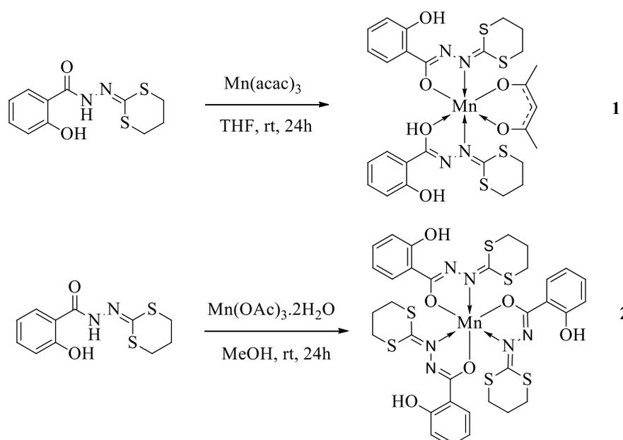
**Scheme 2:** Synthesis of complexes  $\text{Mn}^{\text{III}}(\text{acac})(\text{HL})_2$ (**1**) and  $\text{Mn}^{\text{III}}(\text{HL})_3$ (**2**).
