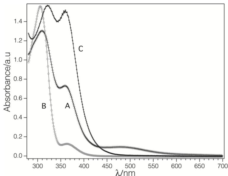
**Figure 14:** Absorption spectra of A)  $\text{Fe}_2^{\text{III}}\text{L}$ , B)  $\text{Fe}^{\text{II}}/\text{H}_4\text{L}$  obtained after light exposure of  $\text{Fe}_2^{\text{III}}\text{L}$ , and C)  $\text{FeCl}_3$ . All solutions are about 1 mM in DMF.
