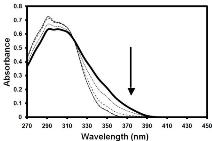
**A3:** Absorbance changes due to the addition of HCl
