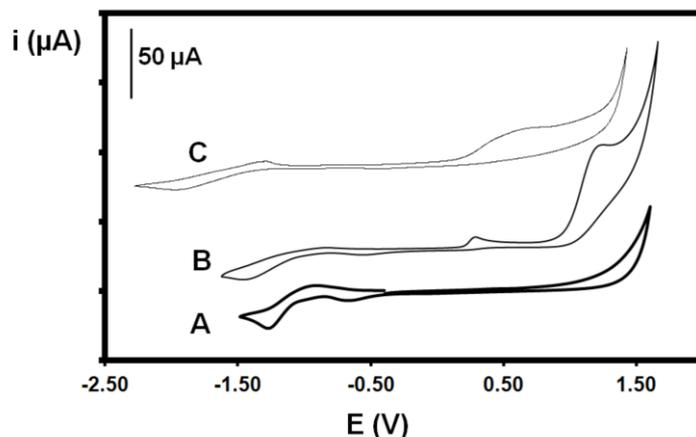
**A 6:** Cyclic voltammograms of A)  $H_4L$ , B)  $H_2L'$  and C)  $H_4L''$  :  $C = 5\text{mM}$ , Pt working electrode, Pt pseudo reference electrode,  $TBAPF_6 = 150\text{mM}$ ,  $\nu = 0.1\text{V}\cdot\text{s}^{-1}$
