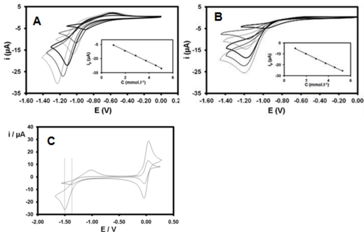
**A 8:** Cyclic voltammograms of A)  $H_4L$  and B)  $H_2L'$  for different concentrations: 1, 1.95, 2.85, 3.72, 4.54 and 5 mM. C) Cyclic voltammogram of  $H_4L$  for 1 mM and 5 mM with ferrocene to calibrate the potentials. DMF, Pt working electrode, Pt pseudo reference electrode,  $TBAPF_6 = 150$  mM,  $v = 0.1V.s^{-1}$ , (insert:  $I_p$  vs.  $C$ )
