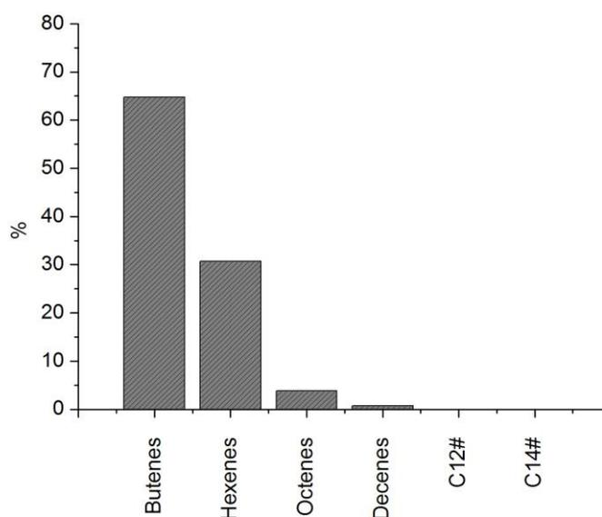
**Figure 7:** Product distribution in the oligomerization of ethylene using **2**/AlEtCl<sub>2</sub> catalytic mixture.
