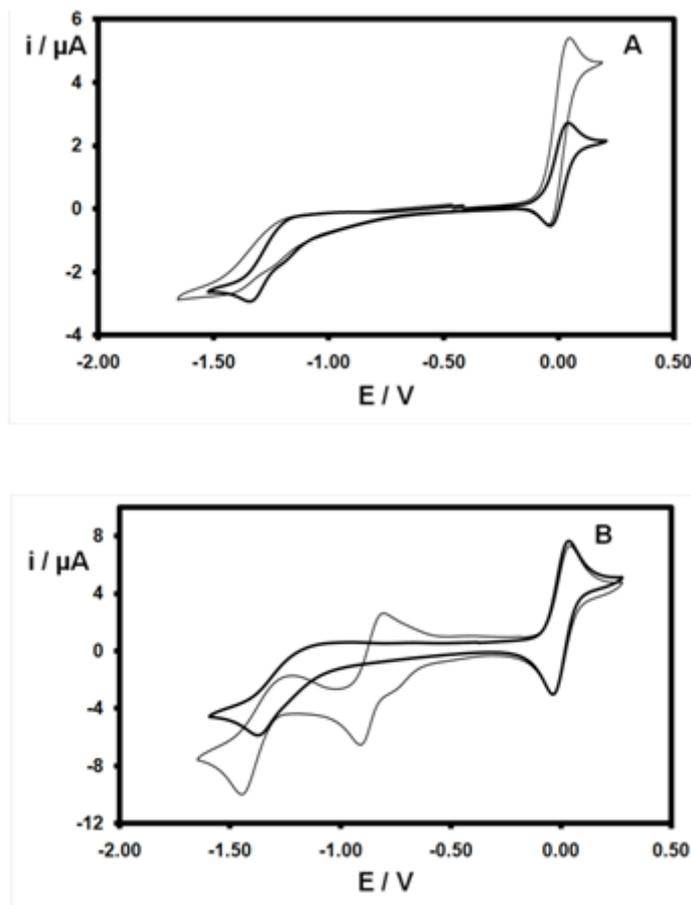
**A 10:** A)  $H_4L$  (thick line) and  $H_2L'$  (thin line) 1 mM,  $\nu = 0.02 \text{ V.s}^{-1}$ .
