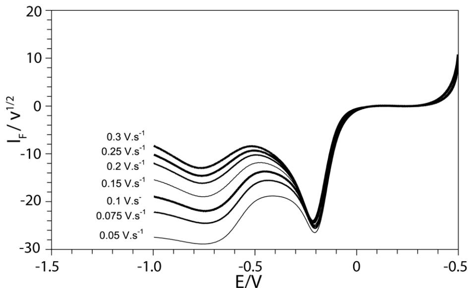
**Figure 13:** Half cyclic voltammograms of  $2\text{FeCl}_3$  and  $\text{H}_4\text{L}$  1 mM at different scan rates in DMF ( $\text{TBA}(\text{PF}_6) = 0.15 \text{ M}$ ). Working electrode: glassy carbon.  $I_F$  is the Faradic current obtained after subtracting the capacitive current.
