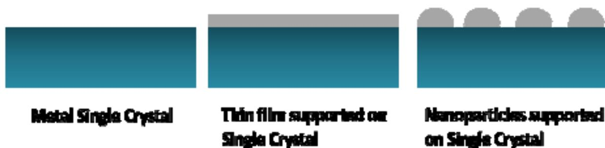
Figure 1.9 Scheme of model catalyst systems
