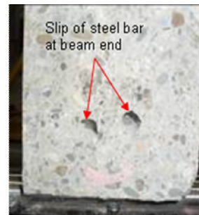
Figure 11. Failure modes of (a) corroded beam A2CL2-B; (b) corresponding control beam
