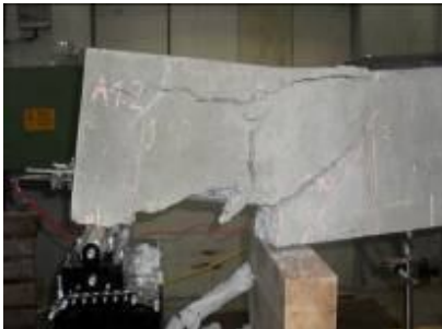
Figure 11. Failure modes of (a) corroded beam A2CL2-B; (b) corresponding control beam
