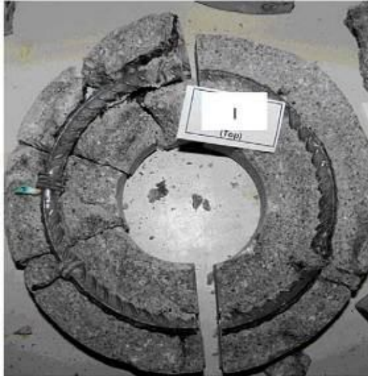
Fig.III-28. Spread of corrosion along the rebar-concrete interface (duration 500 days) a) from a 28 \mu\text{m} opening crack; b) from a 280 \mu\text{m} opening crack [22]
