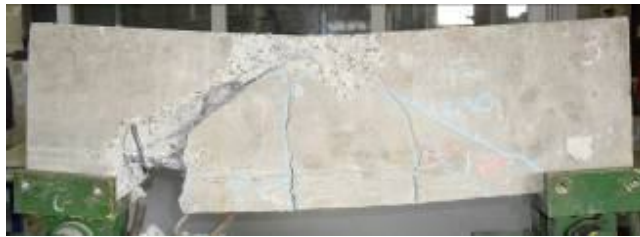
Figure 13. Failure modes of (a) deep corroded beam A2CL2-A; (b) corresponding deep control beam
