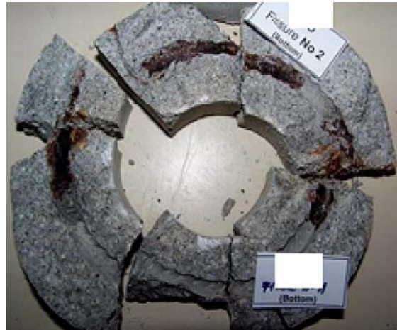
Fig.III-28. Spread of corrosion along the rebar-concrete interface (duration 500 days) a) from a 28 \mu\text{m} opening crack; b) from a 280 \mu\text{m} opening crack [22]
