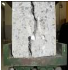
Figure 13. Failure modes of (a) deep corroded beam A2CL2-A; (b) corresponding deep control beam
