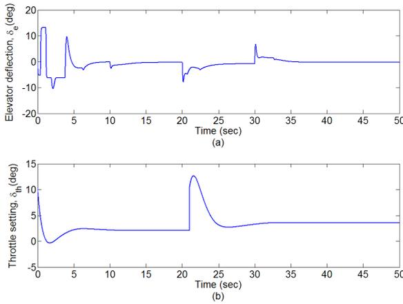
Figure 5.5: Control inputs: elevator deflection  $\delta_e$  (a) and throttle setting  $\delta_{th}$  (b) for FC1.
