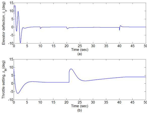
Figure 5.13: Control inputs: elevator deflection  $\delta_e$  (a) and throttle setting  $\delta_{th}$  (b) for FC3.
