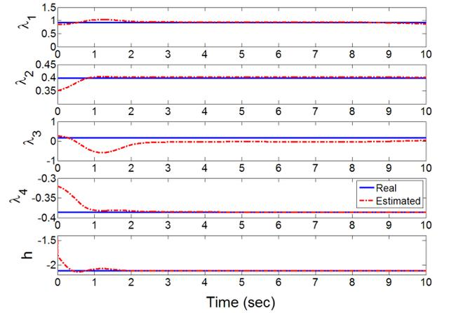
Figure 5.10: Controller parameters estimation related to FC2.
