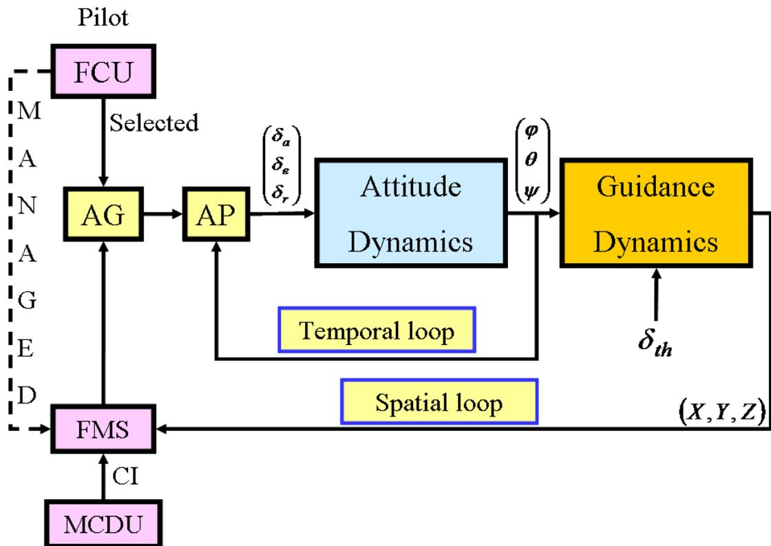
Figure 7.2: Control synoptic scheme
