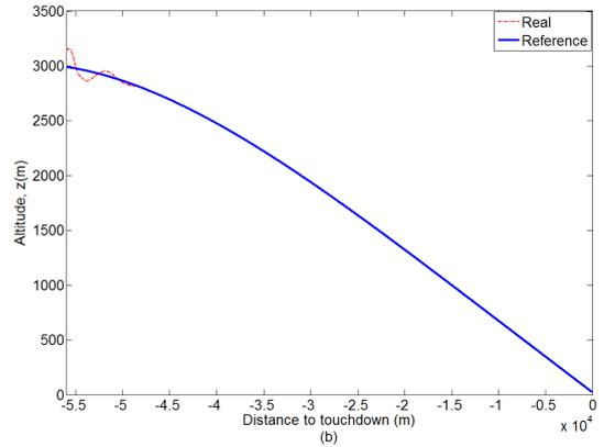
Figure 7.4: Altitude trajectory tracking performance by time NDI (No wind).
