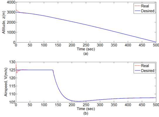
Figure 6.2: Altitude and airspeed tracking performances by NDI.
