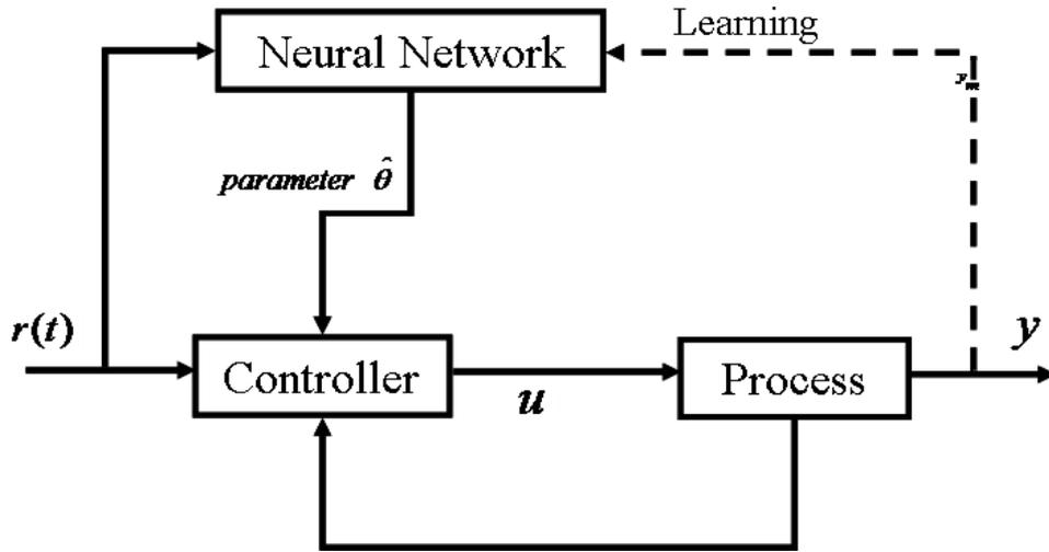
Figure 4.8: Bloc diagram of neural adaptive control
