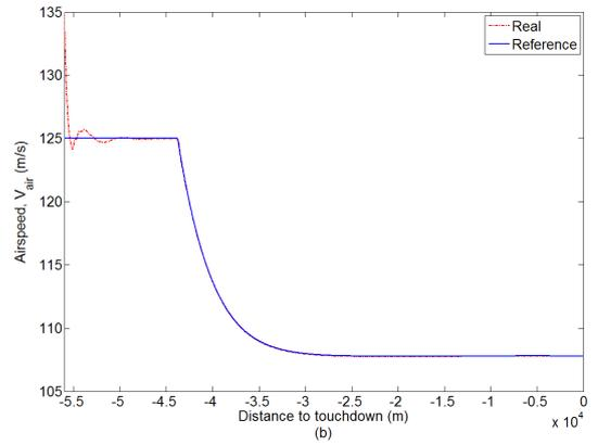
Figure 7.8: Airspeed profile tracking performance by time NDI (No wind).
