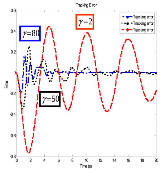
Figure 4.11: Tracking error evolution according to gain adaptation.
