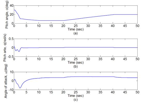
Figure 5.12: Pitch angle (a), pitch rate (b) and angle of attack (c) evolution for FC3.
