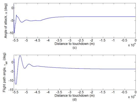
Figure 7.10: Angle of attack and flight path angle evolution with time NDI (c,d), (No wind).
