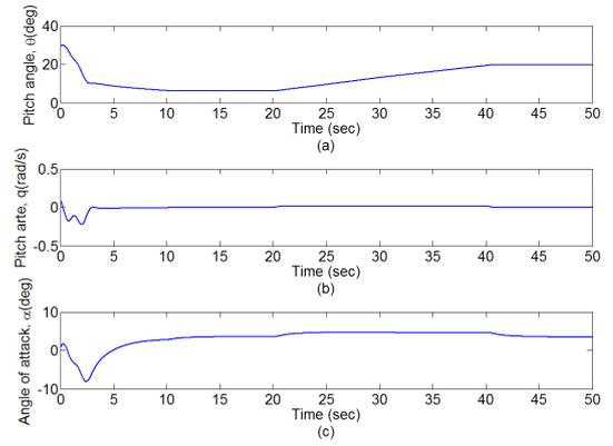
Figure 5.16: Pitch angle (a), pitch rate (b) and angle of attack (c) evolution for FC4.
