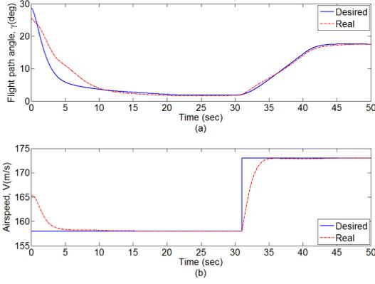
Figure 5.7: Flight path angle (a) and airspeed (b) tracking performances for FC2.
