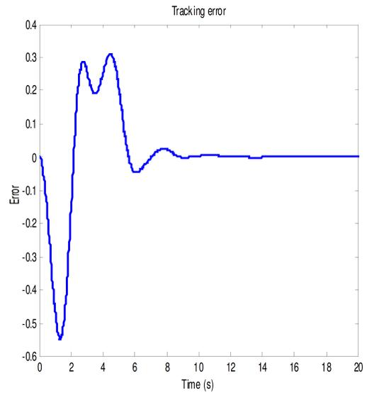
Figure 4.19: Tracking error evolution according to gain adaptation.
