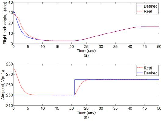
Figure 5.11: Flight path angle (a) and airspeed (b) tracking performances for FC3.
