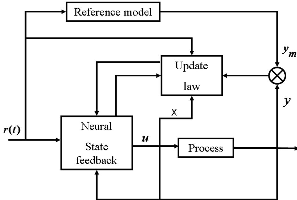
Figure 4.9: Full state-based adaptive neural control structure
