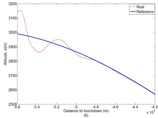
Figure 7.6: Initial altitude tracking by time NDI (No wind).
