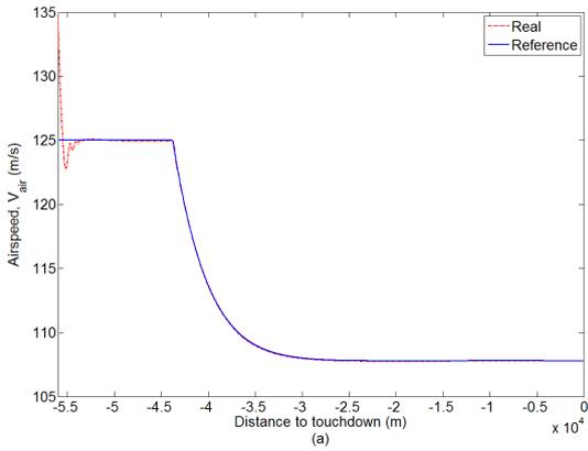
Figure 7.7: Airspeed profile tracking performance by space NDI (No wind).
