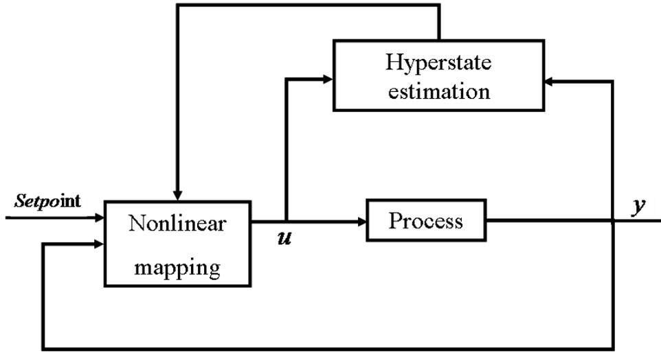
Figure 4.7: Bloc diagram of dual adaptive control
