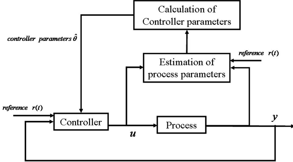
Figure 4.2: Bloc diagram of indirect adaptive control structure
