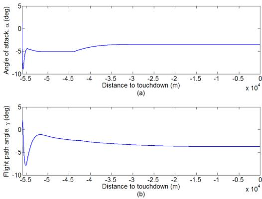
Figure 7.9: Angle of attack and flight path angle evolution with space NDI (a,b), (No wind).
