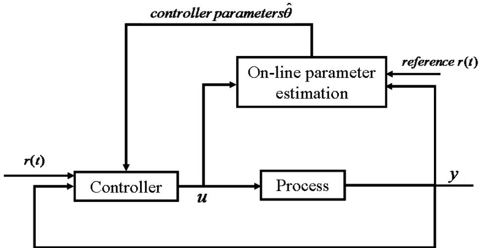
Figure 4.3: Bloc diagram of direct adaptive control structure
