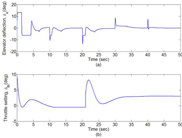
Figure 5.17: Control inputs: elevator deflection  $\delta_e$  (a) and throttle setting  $\delta_{th}$  (b) for FC4.
