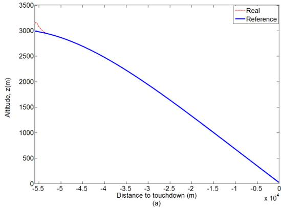
Figure 7.3: Altitude trajectory tracking performance by space NDI (No wind).
