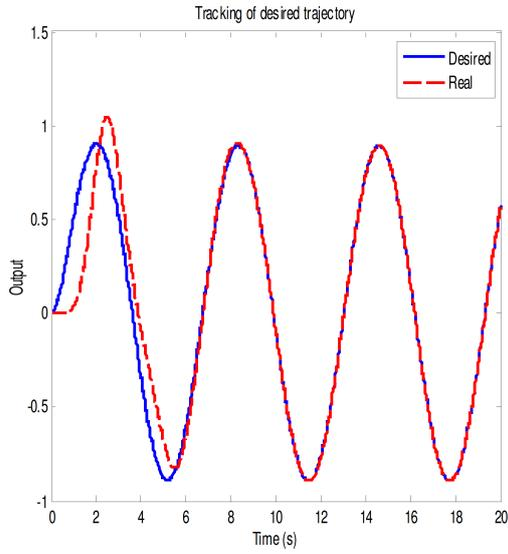
Figure 4.18: MRAC Trajectory tracking performance (MIT rule,  $\gamma = 9$ ).
