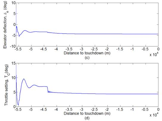
Figure 7.12: Control inputs with time NDI (c,d), (No wind).
