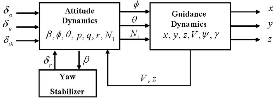
Figure 6.5: Aircraft piloting/Guidance system structure
