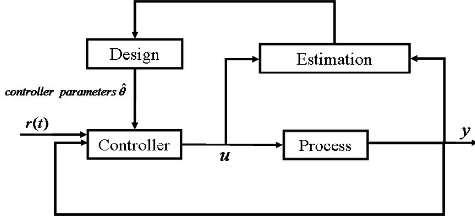
Figure 4.6: Bloc diagram of indirect adaptive self-tuning control
