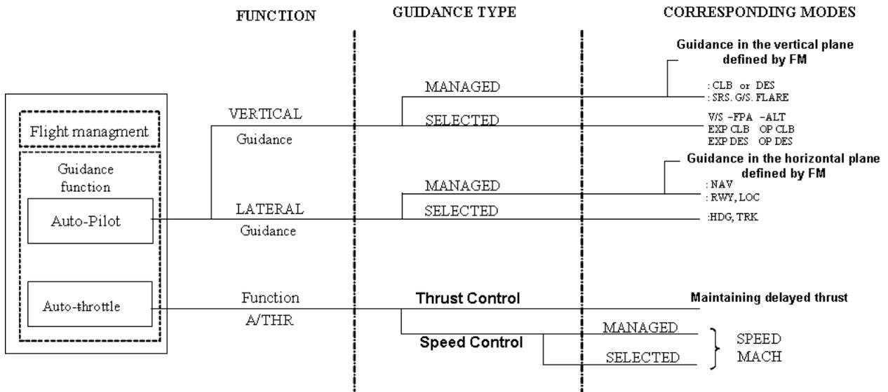
Figure 3.4: Actual guidance types and corresponding modes
