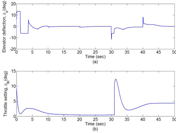
Figure 5.9: Control inputs: elevator deflection  $\delta_e$  (a) and throttle setting  $\delta_{th}$  (b) for FC2.
