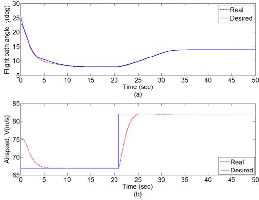
Figure 5.3: Flight path angle (a) and airspeed (b) tracking performances for FC1.
