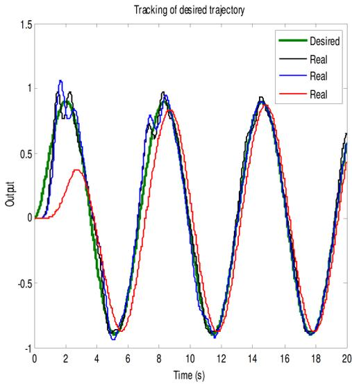
Figure 4.14: MRAC Trajectory tracking performance (MIT rule).
