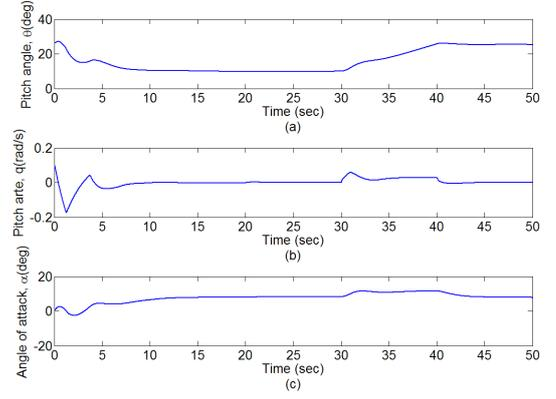
Figure 5.8: Pitch angle (a), pitch rate (b) and angle of attack (c) evolution for FC2.
