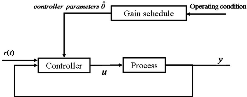
Figure 4.4: Bloc diagram of system with gain scheduling
