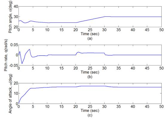
Figure 5.4: Pitch angle (a), pitch rate (b) and angle of attack (c) evolution for FC1.
