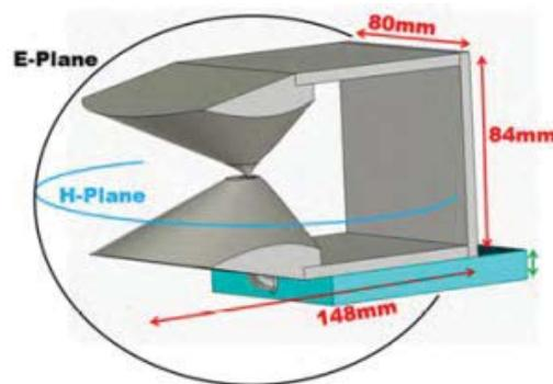
Figure 17 : Antenne Shark [52]
