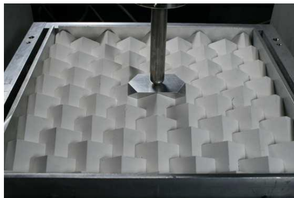
Figure 2.9: Interlocked segmented material made of topologically interlocked cubes. Taken from [DUG13].
