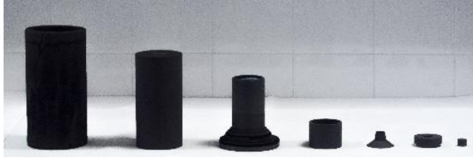
Figure 2.3: The crucible Matryoshka. The parts shown are (from left to right): Thermal insulation, heating element with top cover, powder crucible on base, spacer, cone, sample holder and plug.
