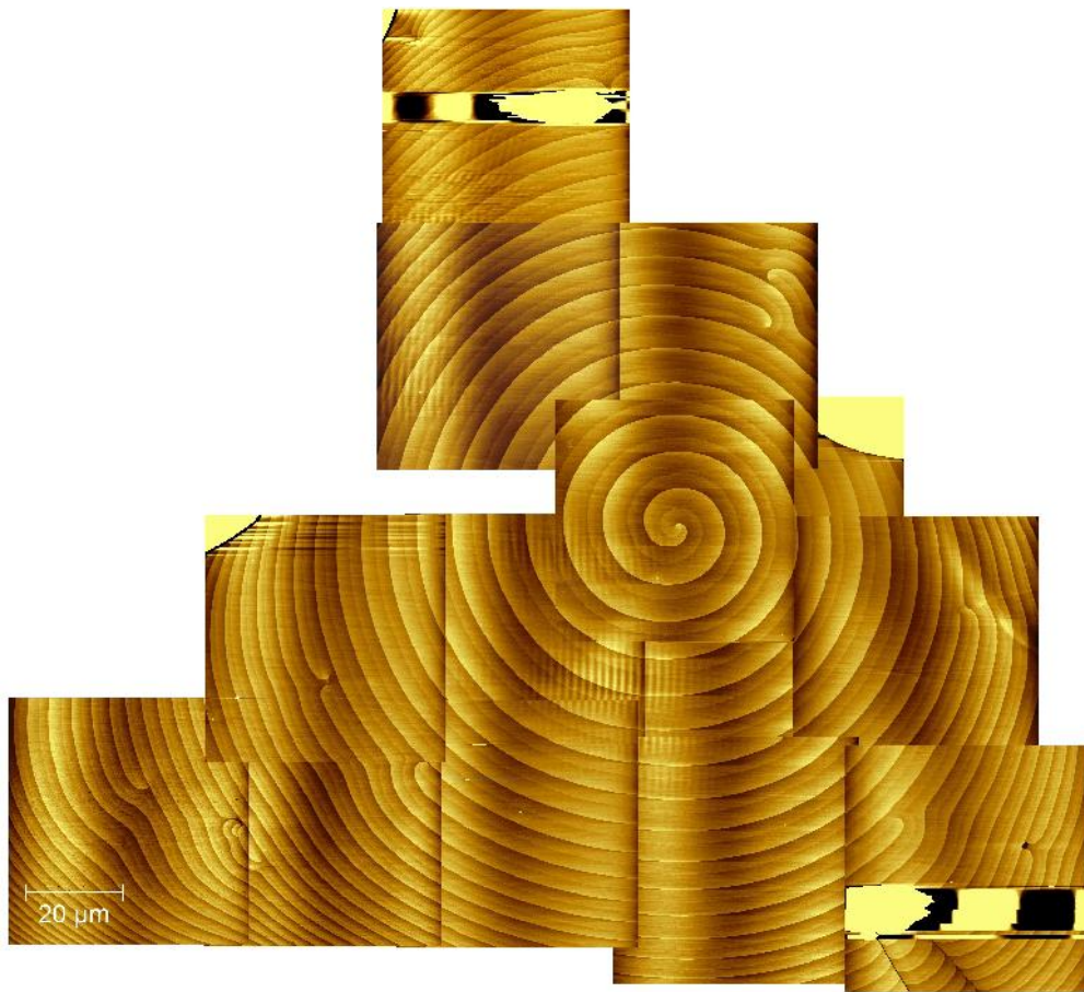
Figure 3.36: A dissociated spiral grown on a Lely seed. The dissociation is maintained over the whole spiral.
