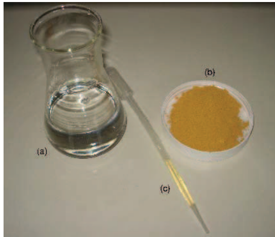
Figure 2.3: Three compounds used in the oil-film mixture: (a) paraffin oil, (b) yellow powder and (c) oleic acid
