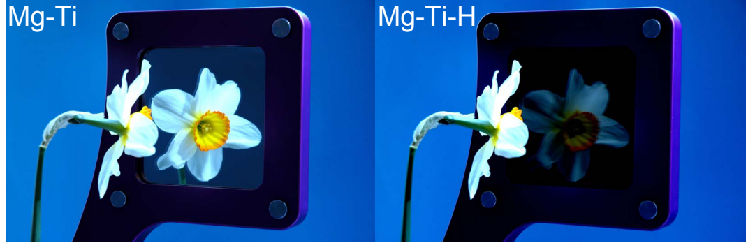
FIGURE 6.1 – Appearance of a 200 nm thick Mg_{70}Ti_{30} film covered with 10 nm of Pd before (left) and after (right) exposure to 10^5 Pa of a 4% H_2 in Ar mixture at room temperature. The pictures are taken from the substrate side. [176]
