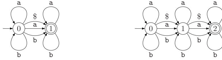
FIGURE 4.3: The cPFT T|a and T|ab of Figure 4.2 represented in the form of automata.
