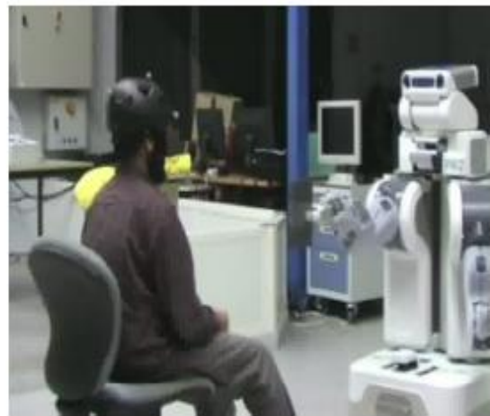
(b) Robot extends arm to handover the object
