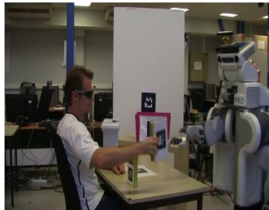
(d) Finally, robot finishes the motion and human hands over the object
