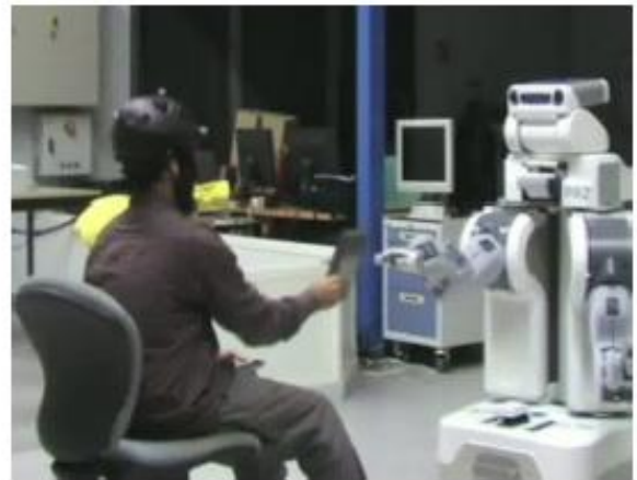
(d) Robot on detecting human intention to take the object, releases the object
