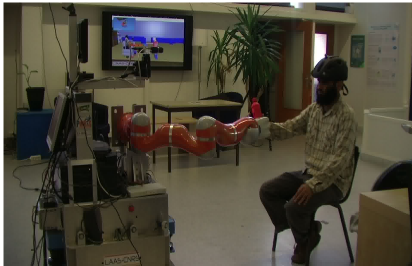
Figure 6.4: Handing over an object to a person: The state observations received and the action selected by the CDM over time is shown here. Initially, the human state is sitting and looking at the robot and the object is with the robot (actual observations starts after 1st second). CDM selects the extend action, moves arm to a give position. When the robot hand state changes to Ready , on detecting the human grabbing the object, a Release action follows and object is then inferred to be with the human.
