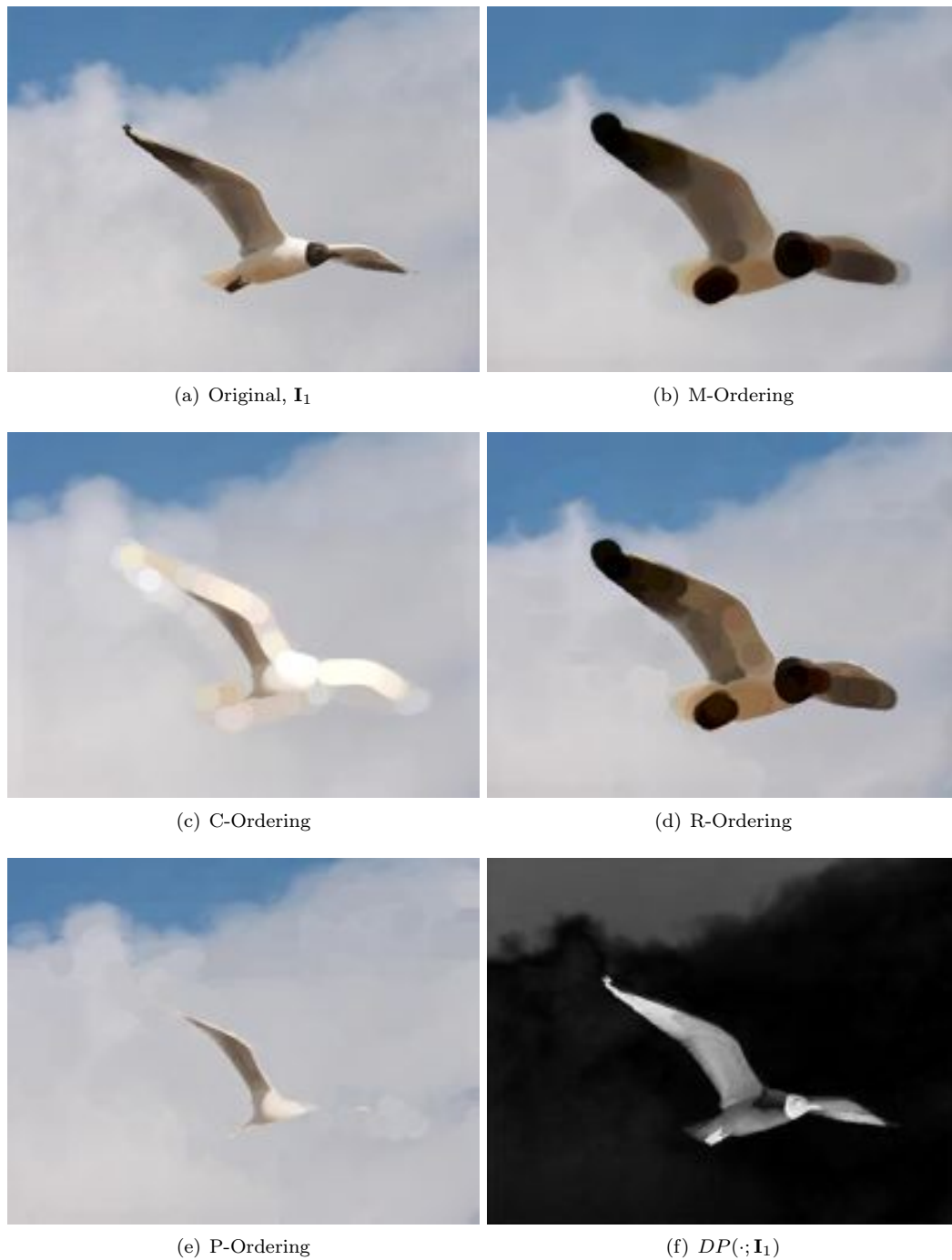
Figure 6.3: Example of different vector morphology operator in the “White-bird” colour image. Erosions by a disk of radius 10 in the family of orders proposed by Barnett (1976) . C-ordering uses the priority red>green>blue. R-ordering is calculated by the saturation component of the colour image. Proposed P-ordering is illustrated in (e).
