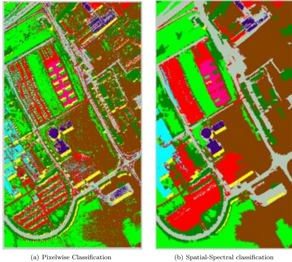
Figure 1.5: Pixelwise and spatial-spectral classification. The aim of spatial-spectral approaches is integrating contextual spatial information with spectral information to produces more “real” results in the classification stage.
