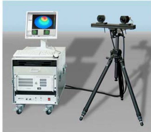
Fig.9. The ARAMIS measurement system set-up in laboratory
