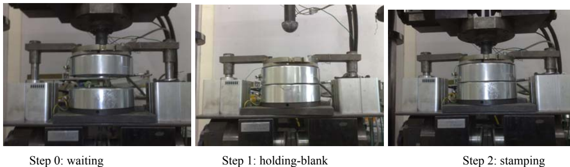
Fig.2. The procedure of the Nakazima stamping tests
