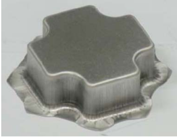
Fig.19. The cross - shaped cup deep drawing specimen and the schematic view of tools.
