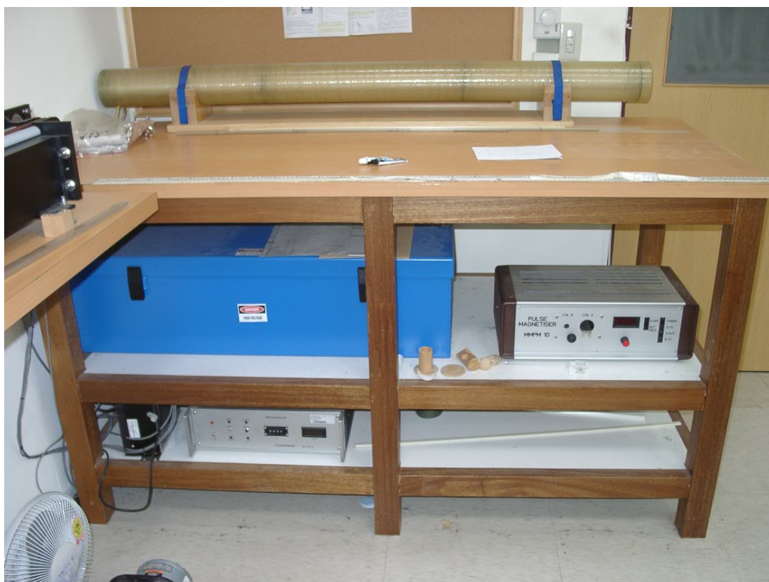
Fig. 2-5: The IRM of the samples was acquired from 25 mT up to 950 mT by using a 2G cryogenic magnetometer.
