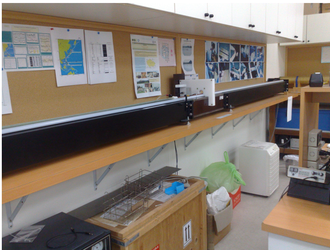
Fig. 4-2: Photo of Bartington MS3 magnetic susceptibility system mounted on an ASC auto-tracking rail in IES, Academia Sinica.
