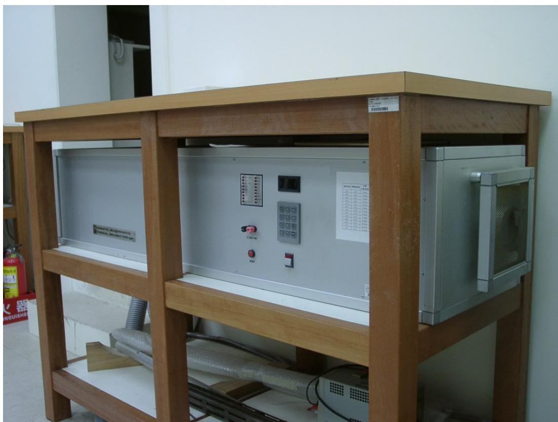
Fig. 2-4: The stepwise heating temperature is from 100°C up to 600°C by using the MMTD80 thermal demagnetizer.
