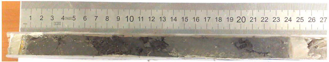
Fig. 2-2: Photo of one U-channel in this study. The U-channel is a plastic box of 2 cm \times 2 cm with \sim 20 cm long.
