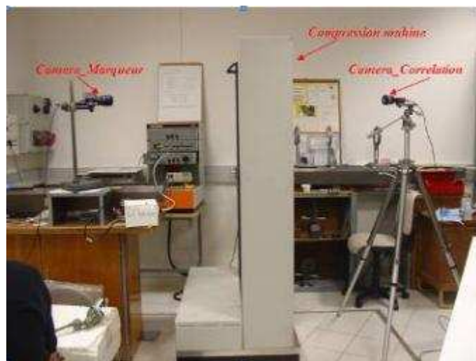
Figure III.7 : Set-up for test under CCD cameras
