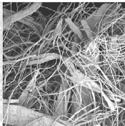
Figure I.15 : SEM images of Wood/PES fiberboard - longitudinal section of 2700 \times 2700 \mu m^2 [10]
