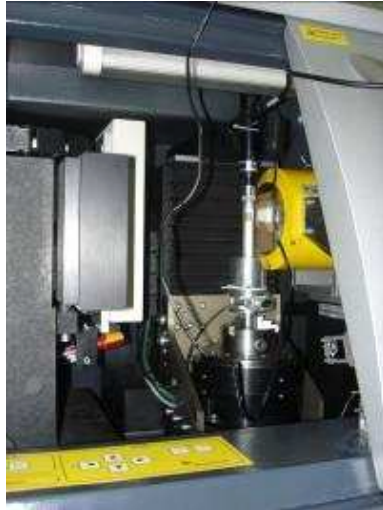
Figure III.9 : Schematic image of Nanotom Phoenix X-ray scanner, developed in laboratory for Wood/PES material
