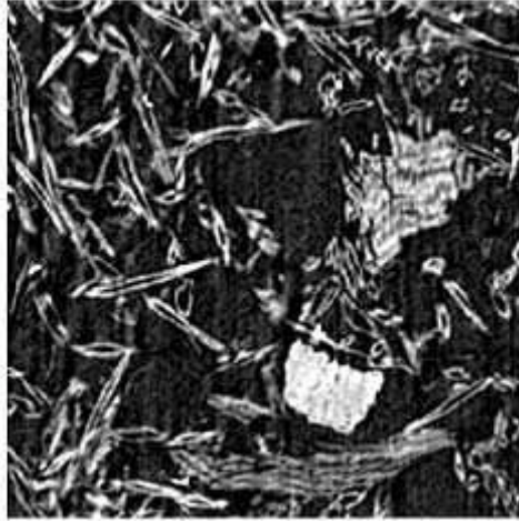
Figure I.17: Longitudinal slice of a microtomographic images of size 400 \times 400 pixels ( 1,9 \times 1,9 \text{ mm}^2 ) at resolution of 4,91 \mu\text{m}/\text{pixel} . ID 19 beam Line, ESRF Grenoble [65]
