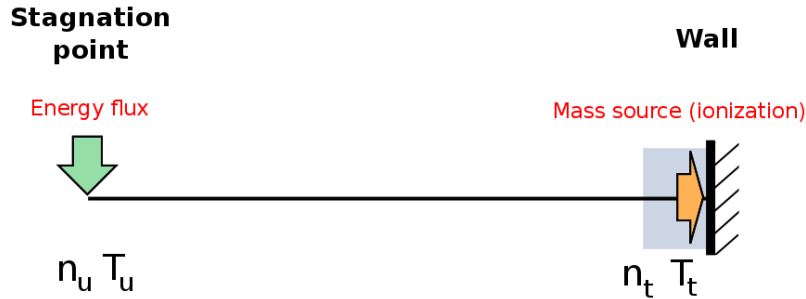
Figure IV.3: 2-points model configuration. The upstream point is located at the stagnation point. The energy source is located at the upstream point whereas the mass source due to recycling is located near the wall
