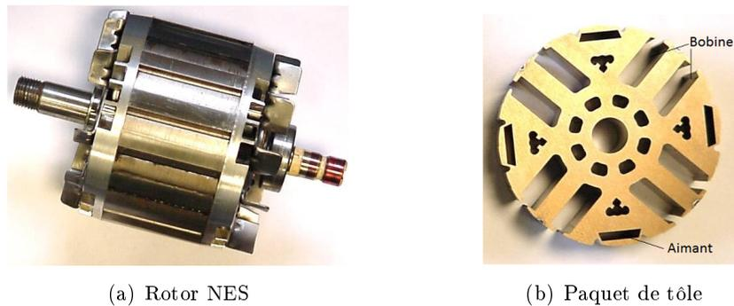
FIGURE I.8 – Prototype NES (new electrical structure) [63]
