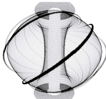
Fig. 2.7 The predicted structure of an ELM in the MAST tokamak plasma geometry, based on the nonlinear ballooning mode theory [25]
