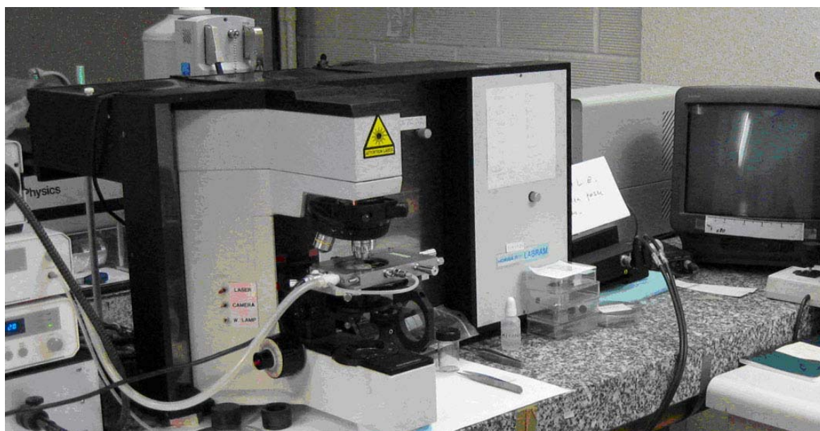
Figure I-8 Photograph of Labram micro-Raman spectrometer (Dilor/Jobin-Yvon/Horiba, USA).
