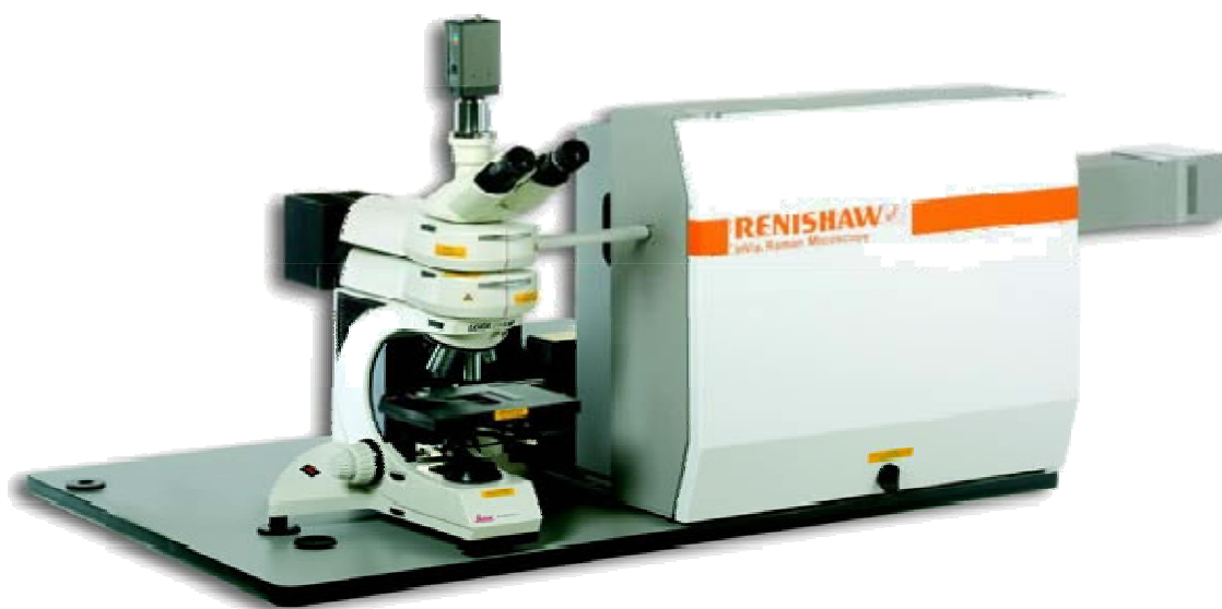
Figure I-9 Photograph of micro-Raman spectrometer (Renishaw, UK)
