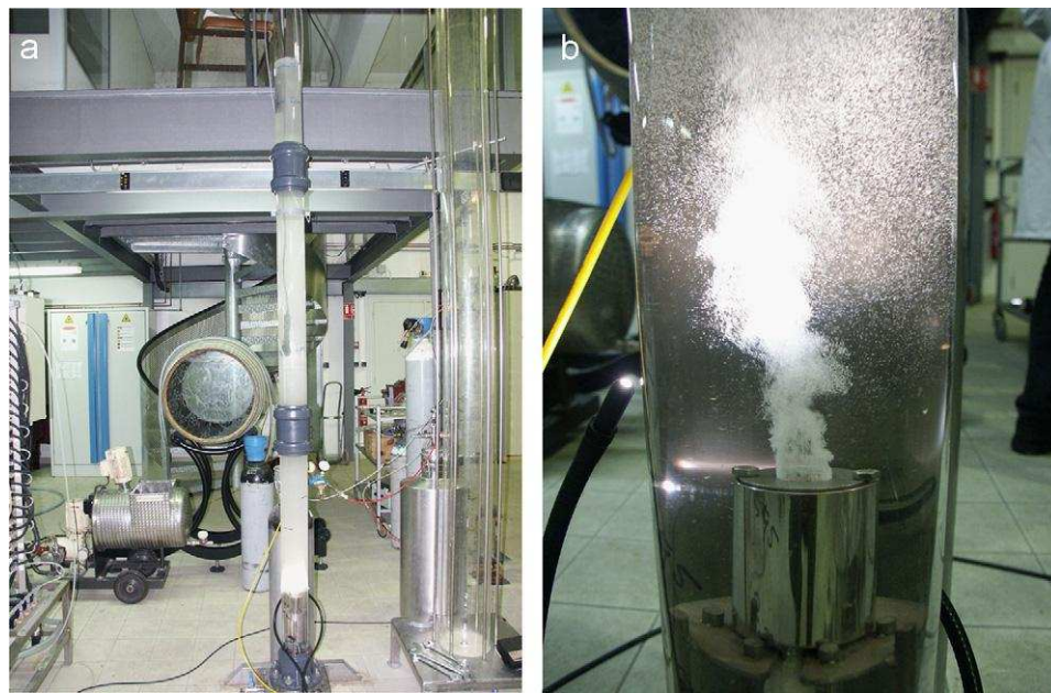
Fig. 1. (a) General view of the experimental bubble column. (b) Detailed view of the ceramic gas distributor.
