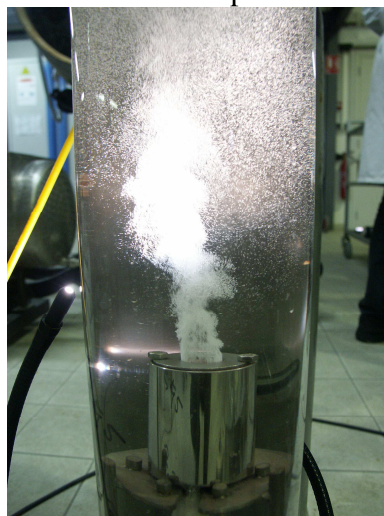
Fig. 3b. Detailed view of gas diffuser
