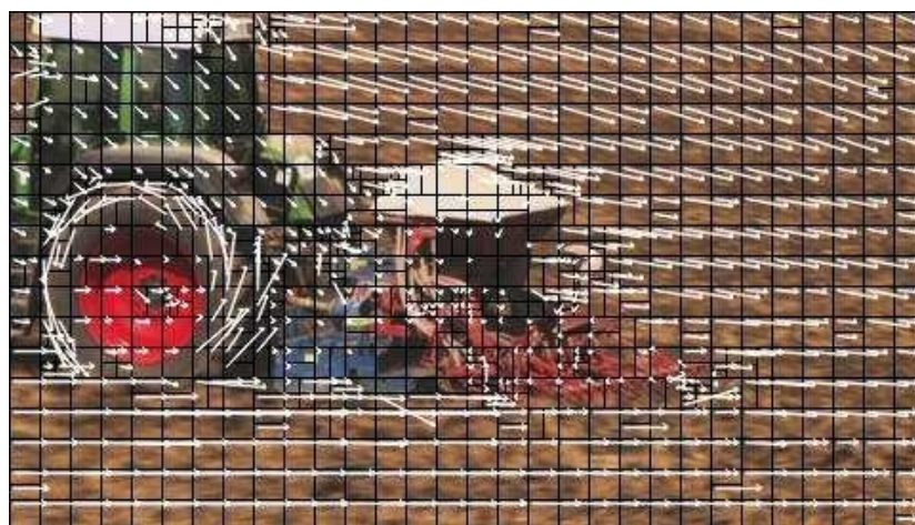
Figure 2.8: Example of MBs and the associated MVs in a H.264/AVC stream. Original sequence ©Taurus Media Technik
