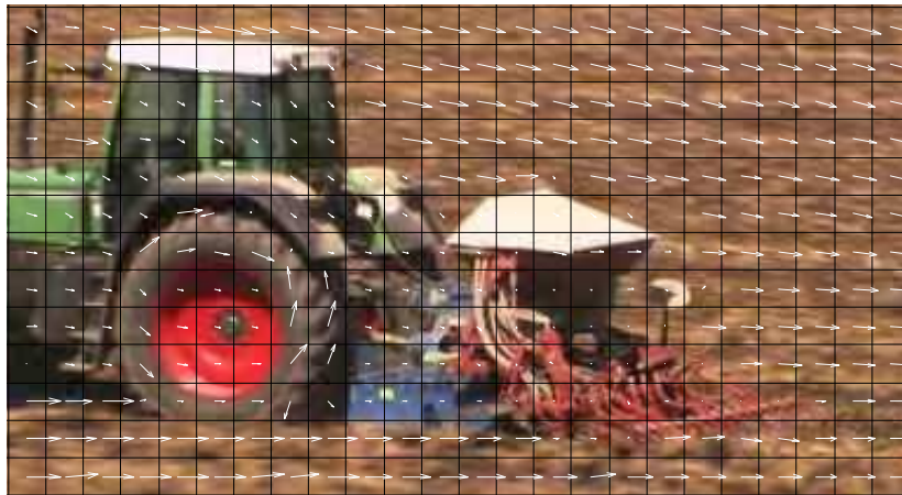
Figure 2.4: Example of MBs and the associated MVs in a MPEG-2 stream. Original sequence ©Taurus Media Technik
