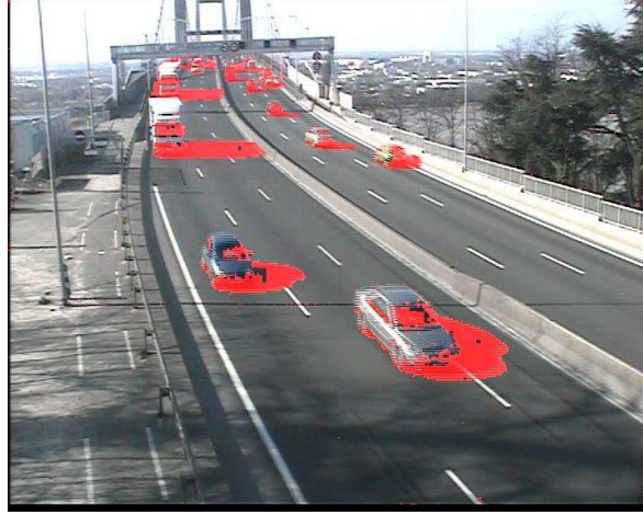
Figure 4.8: Shadow detection result. Shadow pixels are marked in red
